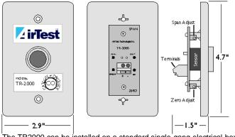
The TR2000 can be installed on a standard single-gang electrical box. A 2" deep PCV box is also provided with the sensor.
